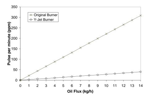
Figure 7- Oil flux in function of the each burner pulse per minute.
