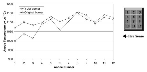
Figure 4- Anode temperature by L<sub>c</sub> method
