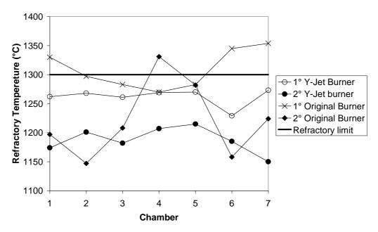
Figure 5- Chamber refractory brick temperature below burners
