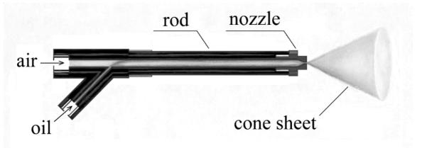
Figure 1- The Y-Jet Atomizer and its assumed Conical Sheet.
