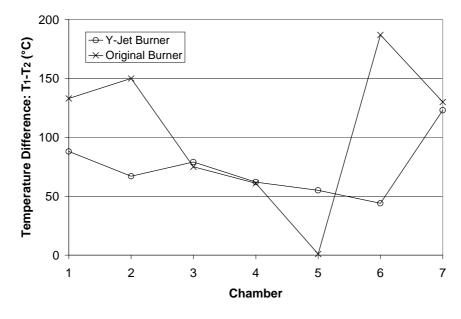
Figure 6- Temperature differences between areas of each chamber.
