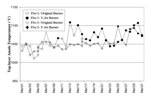
Figure 3- Calcination Temperature of the Anodes from the Top-Layer.
